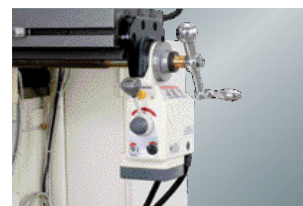
Automatic x-feed 0–900 mm/min, with limit switches and quick motion button
