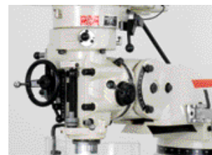
Head swivels \pm 90^\circ and tilts \pm 45^\circ back and forth
