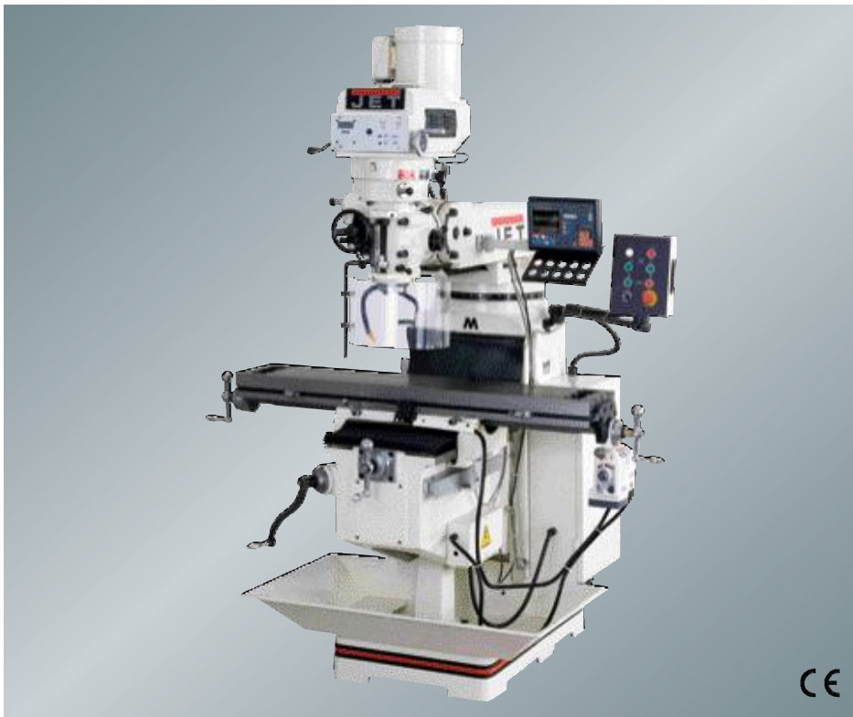
Head swivels \pm 90^\circ and tilts \pm 45^\circ back and forth, adjustable swing 200–680 mm
