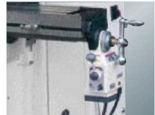
Automatic x-feed 0–900 mm/min, with limit switches and quick motion button
